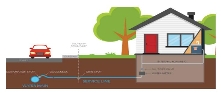
A service line is the pipe that connects a house or business to a water main. The city or township that supplies the water owns the line from the water main to a water shutoff valve called a curb stop, and the homeowner owns the section of service line between the curb stop and the house.
